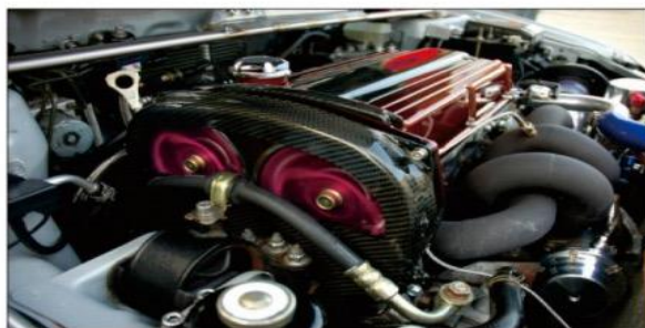
发动机进气管 Engine intake Pipe
